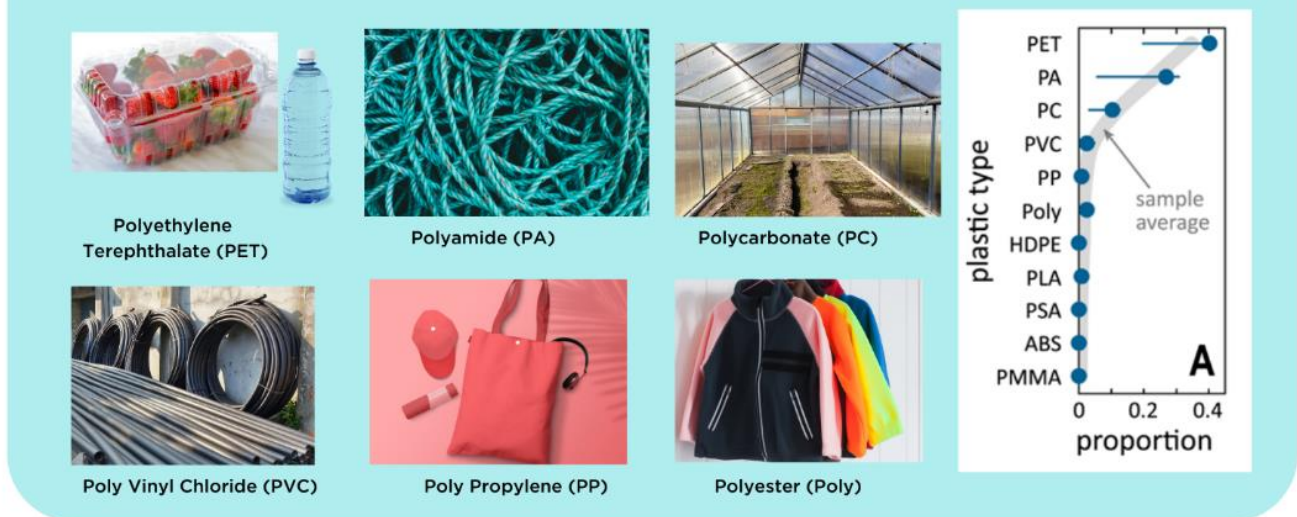
Figure 24. The chemistry of microplastic particles in Monterey Bay were analyzed and about 40% were PET (Choy et al., 2018). Many different products are made from each plastic type, including these examples.
